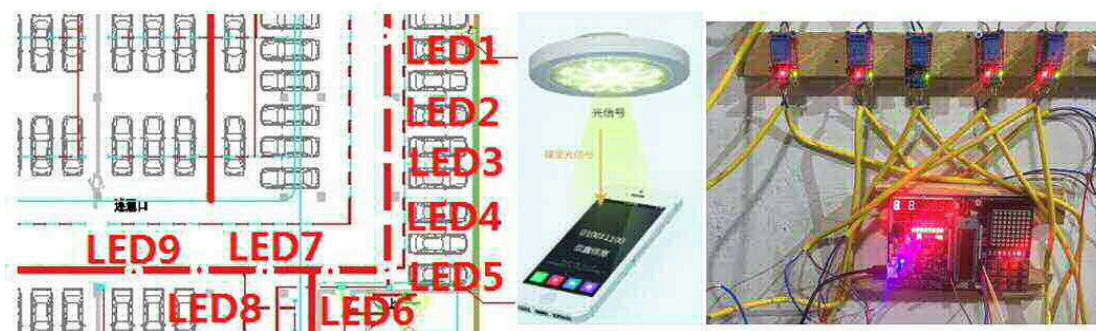
Fig. 4.1.2-1 LED based indoor test bed built by the China University of Mining and Technology, China
