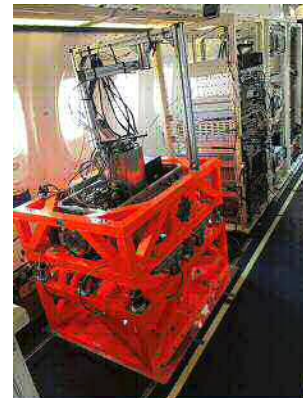
Figure 5b: GIRAFE-2 cold-atom gravimeter (ONERA) during airborne survey in spring 2019.
