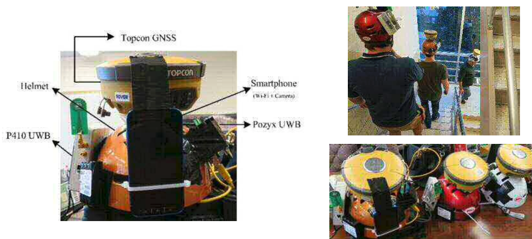
Fig. 4.1.1-3 OSU field campaign 2017. Sensors installed on a helmet (left), indoor-outdoor experiment (top right), and the three of the four helmets used in the research (bottom right).
