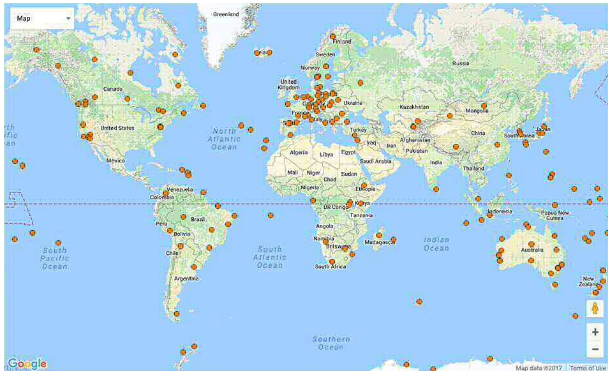
Figure A1.1 GNSS tracking stations in the IGS real-time network
