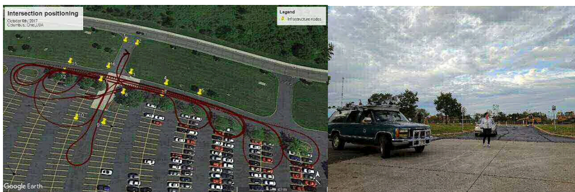
Fig. 4.1.1-2 OSU field campaign 2017. Outdoor vehicle – pedestrian interaction intersection level experiment. Map of the trajectory for one vehicle (left), data collection process and the experimental set-up on field (right)
