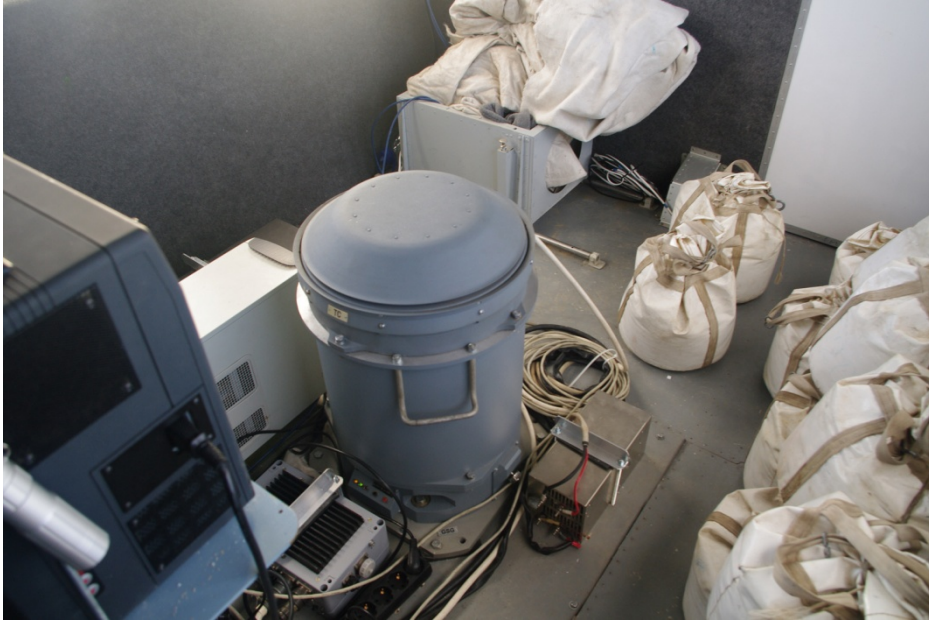
Fig. 2. Relative gravimeter Chekan in a cabin of AU-30.
